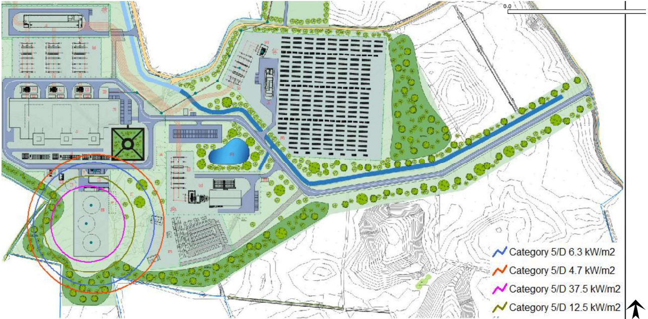
Figure 5-3: Contours for Pool Fire Radiation at category 5/D for Diesel Storage Tank (Northern) Catastrophic Rupture in kW/m 2
