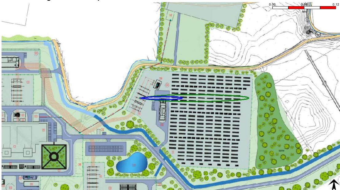
Figure 5-15: Shape of LFL and 1/2 LFL cloud shown for a release at the AGI.
