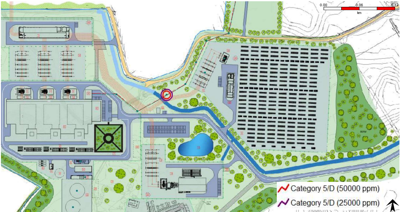
Figure 5-16 Flash Fire at 5/D for both 25000ppm and 50000 ppm for full bore of long pipeline
