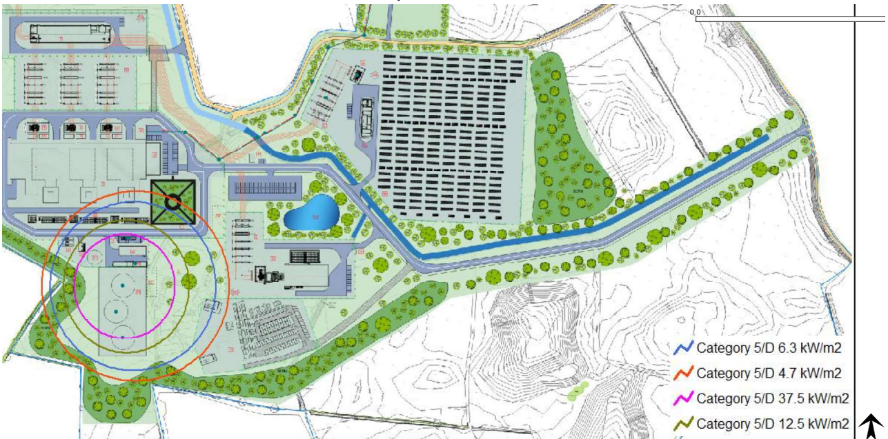
Figure 5-3: Contours for Pool Fire Radiation at category 5/D for Diesel Storage Tank (Northern) Catastrophic Rupture in kW/m 2
